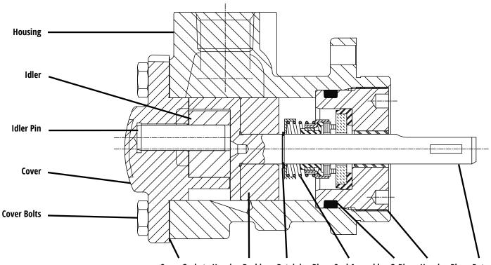
Cover Gasket Housing Bushing Retaining Ring Seal Assembly O-Ring Housing Plug Rotor
