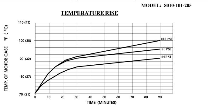
THIS GRAPH IS FOR USE AS A DESIGN GUIDE. IT IS BASED ON RUNNING CONTINUOUSLY WITH AN AMBIENT TEMPERATURE OF  $70^\circ$  F in still air.
