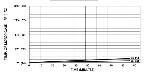
THIS GRAPH IS FOR USE AS A DESIGN GUIDE. IT IS BASED ON RUNNING CONTINUOUSLY WITH AN AMBIENT TEMPERATURE OF  $70^\circ$  F in Still Air.
