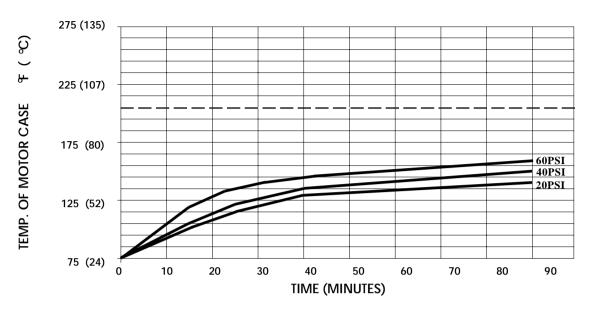
THIS GRAPH IS FOR USE AS A DESIGN GUIDE. IT IS BASED ON RUNNING CONTINUOUSLY WITH AN AMBIENT TEMPERATURE OF 75°F IN STILL AIR. THE THERMAL BREAKER WILL OPEN WHEN THE CASE TEMPERATURE REACHES 205°F.
