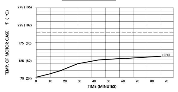
THIS GRAPH IS FOR USE AS A DESIGN GUIDE. IT IS BASED ON RUNNING CONTINUOUSLY WITH AN AMBIENT TEMPERATURE OF 80 ° F IN STILL AIR. THE THERMAL BREAKER WILL OPEN WHEN THE CASE TEMPERATURE REACHES 205 °F.
