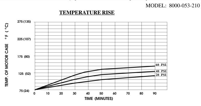
THIS GRAPH IS FOR USE AS A DESIGN GUIDE. IT IS BASED ON RUNNING CONTINUOUSLY WITH AN AMBIENT TEMPERATURE OF 70 ° F IN STILL AIR.
