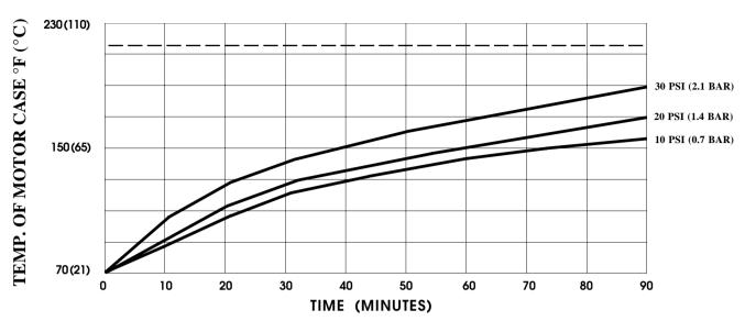
THIS GRAPH IS FOR USE AS A DESIGN GUIDE. IT IS BASED ON RUNNING CONTINUOUSLY WITH AN AMBIENT TEMPERATURE OF 70°F (21°C) IN STILL AIR. --- OPERATIONAL LIMIT.
