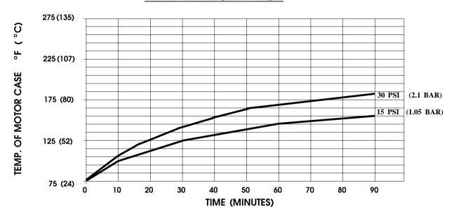
THIS GRAPH IS FOR USE AS A DESIGN GUIDE. IT IS BASED ON RUNNING CONTINUOUSLY WITH AN AMBIENT TEMPERATURE OF 75° F (24°C) IN STILL AIR.
