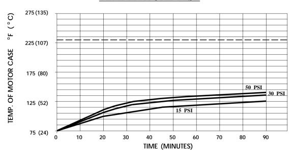
THIS GRAPH IS FOR USE AS A DESIGN GUIDE. IT IS BASED ON RUNNING CONTINUOUSLY WITH AN AMBIENT TEMPERATURE OF 70°F INSTILL AIR. THE THERMAL BREAKER WILL OPEN WHEN THE CASE TEMPERATURE REACHES 230°F.
