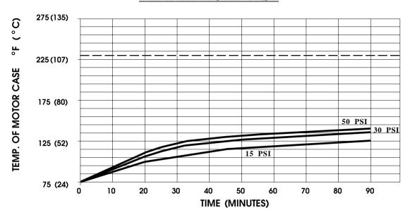
THIS GRAPH IS FOR USE AS A DESIGN GUIDE. IT IS BASED ON RUNNING CONTINUOUSLY WITH AN AMBIENT TEMPERATURE OF  $70^{\circ}$  F IN STILL AIR. THE THERMAL BREAKER WILL OPEN WHEN THE CASE TEMPERATURE REACHES  $230^{\circ}$  F.
