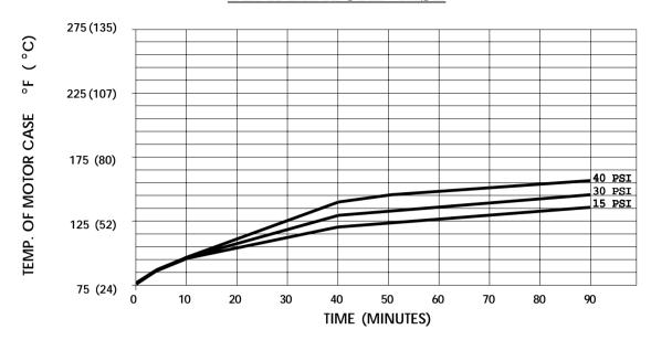
THIS GRAPH IS FOR USE AS A DESIGN GUIDE. IT IS BASED ON RUNNING CONTINUOUSLY WITH AN AMBIENT TEMPERATURE OF 75° F IN STILL AIR. THE THERMAL BREAKER WILL OPEN WHEN THE CASE TEMPERATURE REACHES 280°F.
