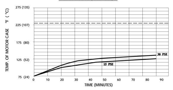
THIS GRAPH IS FOR USE AS A DESIGN GUIDE. IT IS BASED ON RUNNING CONTINUOUSLY WITH AN AMBIENT TEMPERATURE OF  $70^{\circ}$ F INSTILL AIR. THE THERMAL BREAKER WILL OPEN WHEN THE CASE TEMPERATURE REACHES 230 F.
