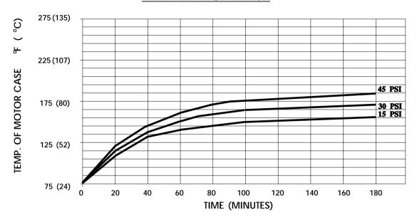
THIS GRAPH IS FOR USE AS A DESIGN GUIDE. IT IS BASED ON RUNNING CONTINUOUSLY WITH AN AMBIENT TEMPERATURE OF 75° F IN STILL AIR.
