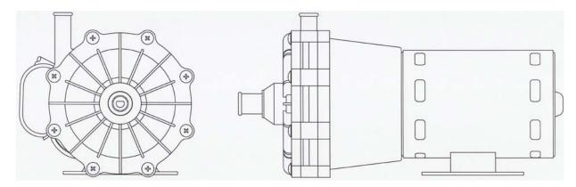
For applications requiring low flow, but when it's necessary to develop pressure. This compact sized corrosion resistant pump has the durability of a centrifugal pump for continuous duty.
