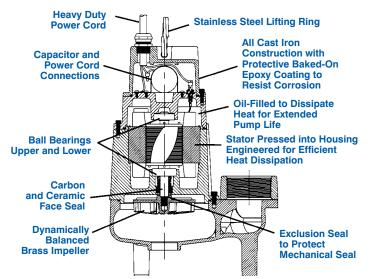
For residential, commercial, industrial and agricultural use. The Model 20S Series sewage ejector pumps handle liquids and solids up to 2" in diameter. Pumps feature 3" FNPT discharge with a maximum head of 77', heavy-duty cast iron construction and stainless steel hardware.
