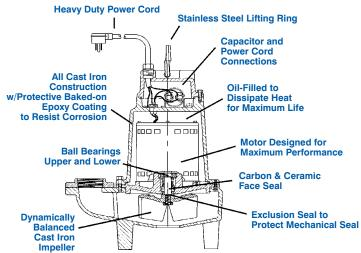
For residential, commercial, industrial and agricultural use. The model 14S Series Wastewater and Sewage Ejector pumps handle liquids and solid waste materials up to 2" in diameter. Pumps feature either a 2" or 3" FNPT discharge with a maximum head of 25', heavy duty cast iron construction and stainless steel hardware.
