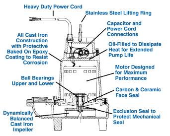
For Residential, Commercial, Industrial and Agricultural use. Pumps feature 2" FNPT discharge with a lift of 50'. Heavy duty cast iron construction and stainless steel hardware.
