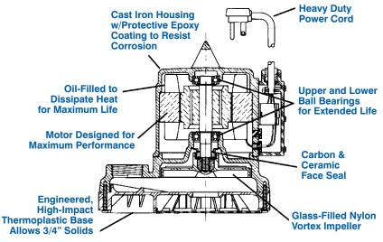
The Model 10E Series De-watering and Effluent pumps are for commercial and light industrial applications. Pumps feature a 1-1/2" discharge, with a lift of 26', ABS base, vortex nylon impeller and glass-filled electrical case.
