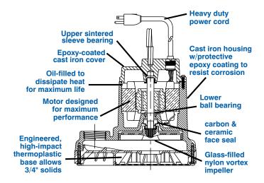
The Model 9E Series De-watering and Effluent pumps are for residential and light to medium commercial use. Pumps feature a 1-1/2" discharge with a lift of 23' and ABS base.
