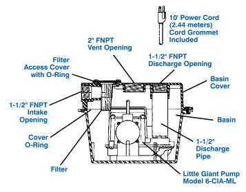
The compact "DRAINOSAUR" removes water from laundry trays, lavatory sinks, wet bar sinks, dehumidifiers, air conditioners (condensate), water softeners, etc. Installs above floor, no need to dig a sump. Unit is pre-assembled and ready-to-install.
