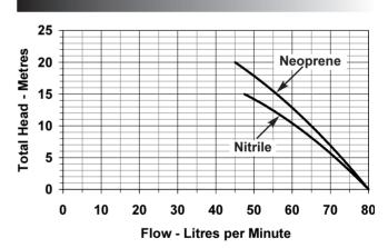
Note: Performance shown is for a new pump, pumping water at 20°C, performance may vary by up to 15%. factory for performance of alternative impeller compounds.
