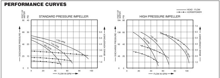
NOTE: Curves show approximate head flow for new pumps with neoprene impeller pumping water. Capacities should be reduced approximately 20% with high pressure EPDM impeller.
