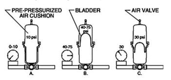
chamber forces water into the system. Pump stays off until minimum pressure is reached. Then pump turns on.
