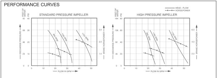
NOTE: Curves show approximate head flow for new pumps with neoprene impeller pumping water. Capacities should be reduced approximately 20% with high pressure EPDM impeller.
