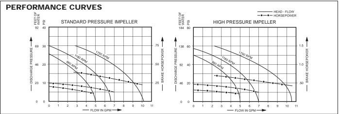
NOTE: Curves show approximate head flow for new pumps with neoprene impeller pumping water. Capacities should be reduced approximately 20% with high pressure EPDM impeller.
