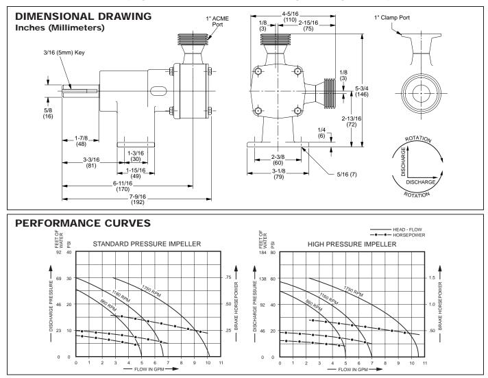
NOTE: Curves show approximate head flow for new pumps with neoprene impeller pumping water. Capacities should be reduced approximately 20% with high pressure EPDM impeller.
