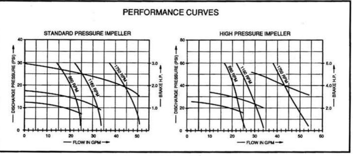
NOTE: Curves show approximate head flow for new pumps with neoprene impeller pumping water.
