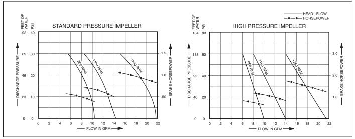
NOTE: Curves show approximate head-flow for new pumps with neoprene impeller pumping water.
