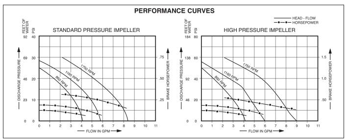
NOTE: Curves show approximate head-flow for new pumps with neoprene impeller pumping water.
