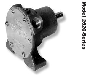
SELF-PRIMING – Primes at low or high speeds. For vertical lift of 10 feet (3.0mm), a minimum of 800 RPM is required. Pump will produce suction lift of up to 22 feet (6.7m) when wetted. BE SURE SUCTION LINES ARE AIRTIGHT OR PUMP WILL NOT SELF-PRIME.
