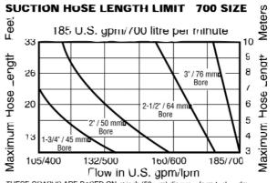
THESE GRAPHS ARE BASED ON: 2 inch (50 mm) diameter farm tank outlet One elbow between suction hose and pump inlet. Farm tank milk level 0.5 ni below pump level on vehicle
