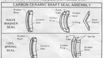
In this pump, either a wave washer seal or coil spring seal may be used. The wave washer is used only if the carbon portion of the seal does not have a coil spring attached.
