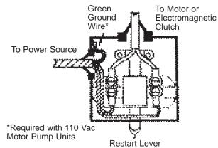
REMOTE RESTART OR AUTOMATIC\* CONTROL SWITCH On electric clutch or motor pump units, a remote restart switch may be installed to eliminate the need to manually activate restart lever.
