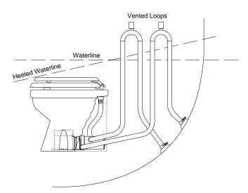
diameter quality waste compatible hose. If discharging overboard, the discharge seacock should be located well aft and above the location of the intake seacock. Connect the discharge hose to the 1" (25 mm) barbed discharge port on the white plastic toilet base. Secure all hose connections with two marine grade S.S. band clamps at each connection.
