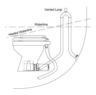
If the toilet is plumbed to an overboard discharge, and is below the vessel's waterline, the discharge plumbing must include a properly positioned vented loop. The vented loop fitting must be secured in a location that remains at least 6-8 inches (15-20 cm) above the waterline at all angles of heel and trim. The maximum discharge head without a notable decrease in pump performance is four feet (1.3 M).
