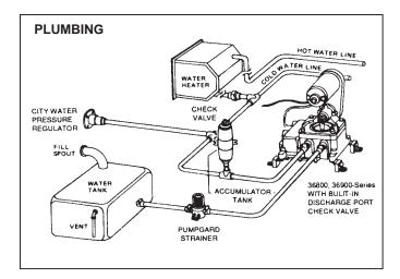
PRESSURE REGULATOR It is recommended that systems having a connection for a city water entry be equipped with a pressure regulating check valve set at approximately 35 psi. This valve automatically regulates the incoming water pressure to avoid damage to pump and plumbing from excessive pressures. Models 44410-Series (Permanent Flush Mount) and 44410-1010 (in-line Hose Type) pressure regulating valves are recommended for this purpose.
