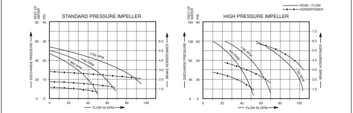
NOTE: Curves show approximate head flow for new pumps with neoprene impeller pumping water. Capacities should be reduced approximately 20% with high pressure EPDM impeller.
