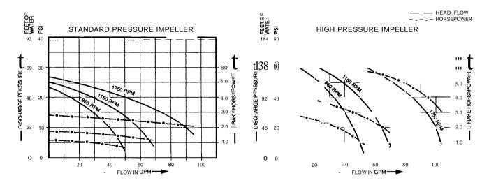
NOTE: Curves show approximate head-flow for new pumps with neoprene impeller pumping water. Capacities should be reduced approximately 10% with nitrile standard pressure impeller and EPDM high pressure impeller.
