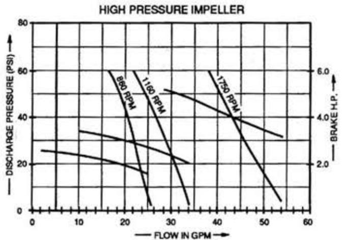
NOTE: Curves show approximate head flow for new pumps with neoprene impeller pumping water.
