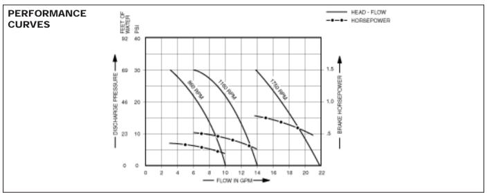
NOTE: Curves show approximate head-flow for new pumps with neoprene impeller pumping water. Capacities should be reduced approximately 10% with nitrile, viton and EPDM impellers. Consult factory for specific performance information.
