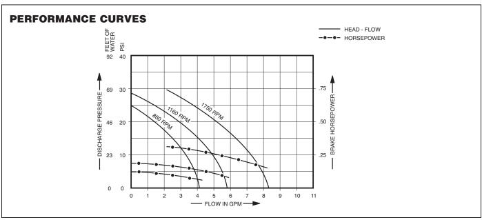
NOTE: Curve shows approximate head-flow for new pumps with neoprene impeller pumping water. Capacities should be reduced approximately 10% with nitrile impeller.
