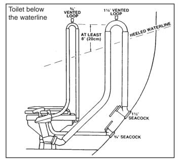
If unfamiliar with proper plumbing requirements for marine toilets, it is recommended that a qualified marine plumbing technician is contacted to do the installation.
