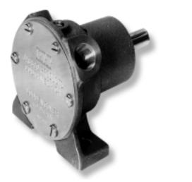
SELF-PRIMING – Primes at low or high speeds. For vertical lift of 10 feet (3.0mm), a minimum of 800 RPM is required. Pump will produce suction lift of up to 22 feet (6.7m) when wetted. BE SURE SUCTION LINES ARE AIRTIGHT OR PUMP WILL NOT SELF-PRIME.
