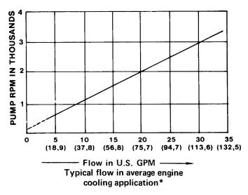
\*Average engine cooling applications have discharge pressures of 10-15 PSI and inlet vacuums of 3-5 inches of mercury.
