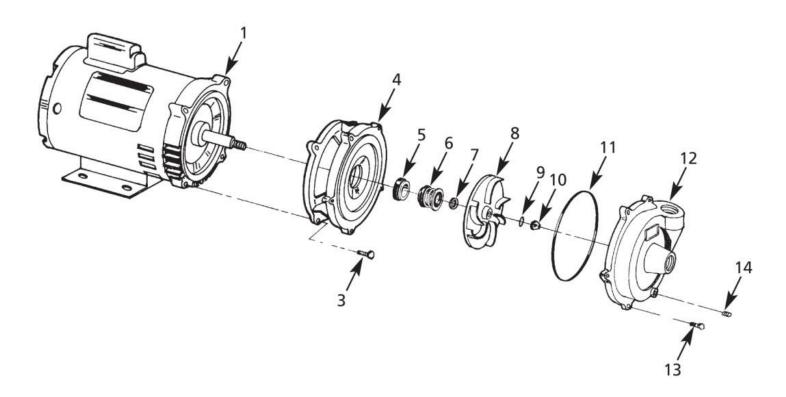
Figure 2 - Repair Parts Illustration
