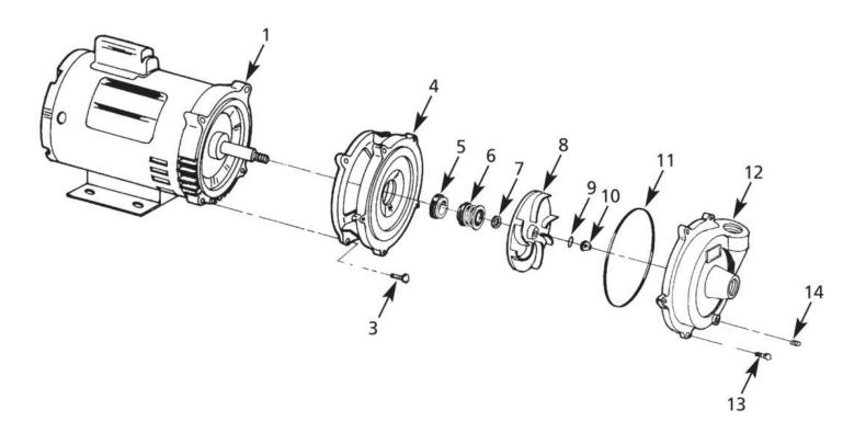
Figure 2 - Repair Parts Illustration
