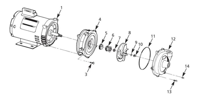
Figure 2 - Repair Parts Illustration
