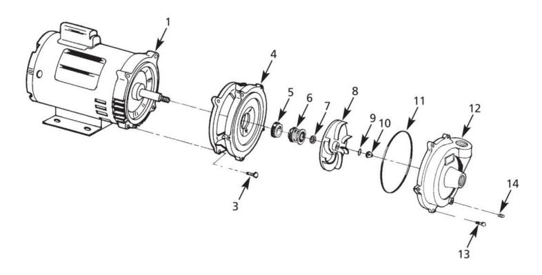
Figure 2 - Repair Parts Illustration
