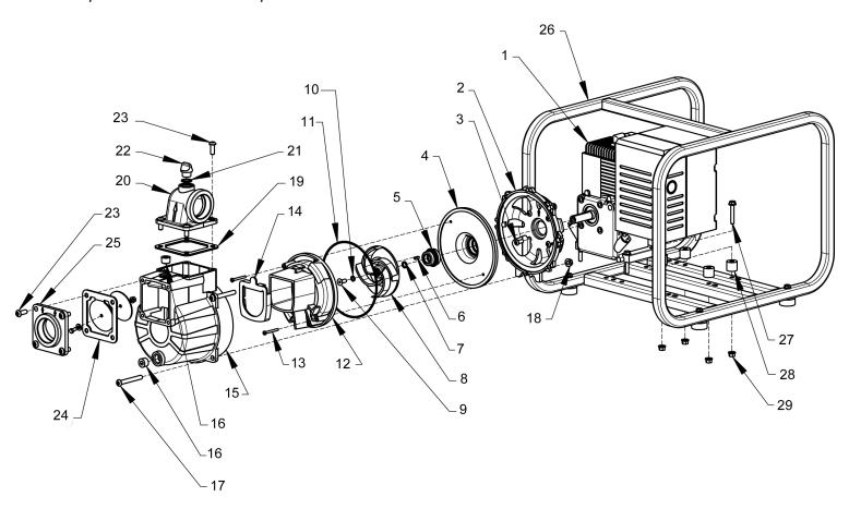
Figure 1 - Repair Parts Illustrations
