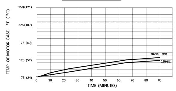
THIS GRAPH IS FOR USE AS A DESIGN GUIDE. IT IS BASED ON RUNNING CONTINUOUSLY WITH AN AMBIENT TEMPERATURE OF 75  $^{\circ}$ F INSTILL AIR. THE THERMAL BREAKER WILL OPEN WHEN THE CASE TEMPERATURE REACHES 230  $^{\circ}$ F.
